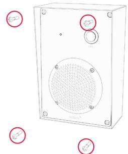
6. Mark the x4 fixing point holes and cable management hole on the mounting surface.
